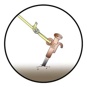
For added security, install cords across the tarp between each pair of grommets and attach these to stakes or securing devices in the ground. This will reduce the size of the gaps between the metal roof and the tarp.
