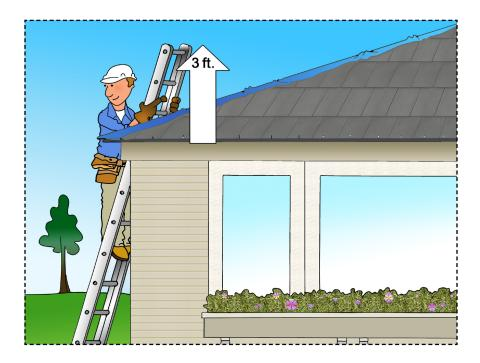
Inspect the roof to make sure all debris is cleared and be careful to avoid any holes in the roof. Do not attempt to cover the roof during wet conditions.
