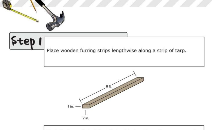
Each furring strip is 6 feet (1.8 m) in length, so if you are covering a small area of damage, one strip may suffice. If you are covering a large area, you may need to abut two or more strips until you have a long enough length of wood.
