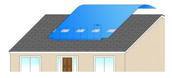
To prevent rust stains, use 8d common galvanized steel nails, and space them 2 feet (60 cm) apart on center.
