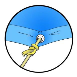
Now anchor the cords to the ground with tent stakes or other suitable securing devices.
