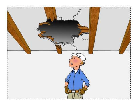
For a temporary repair of joists and rafters, use  $2'' \times 4''$  lumber, cut to size, and install as necessary to provide proper anchorage and support for the temporary plastic roofing and roof decking.
